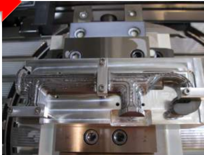
Machined from flat to round cross section.
